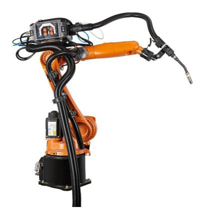
Kemppi offers robotic gun packages both hollow wrist and non-hollow wrist robot arm designs. The perfect welding gun system for robotic arc welding consists of the gun neck with a tip holder, a gas nozzle and a cable assembly. A robotic gun can be mounted on a suitable Kemppi Gun Mount.
