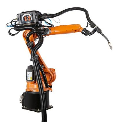
Kemppi offers robotic gun packages both hollow wrist and non-hollow wrist robot arm designs. The perfect welding gun system for robotic arc welding consists of the gun neck with a tip holder, a gas nozzle and a cable assembly. A robotic gun can be mounted on a suitable Kemppi Gun Mount.
